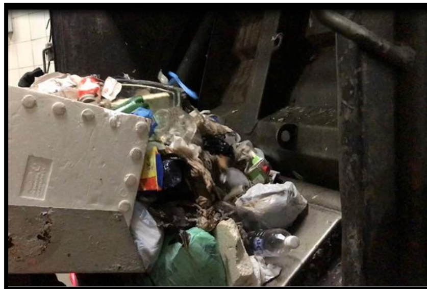
壓縮型垃圾車接收從固定的壓縮機卸出的垃圾 Waste vehicles with rear compactors receive refuse discharged from fixed compactors.
