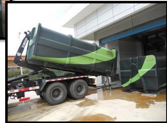
垃圾由翻斗投進固定壓縮機機體 Refuse is transferred into the fixed compaction chamber by the bin lifter or the tipper.
